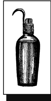
Figure 44—A traditional oil bottle applies liberal amounts of saw lubricant. The hook held the bottle to the log, conveniently within reach.— Now You're Logging , by Bus Griffiths, with permission of Harbour Publishing, Madeira Park, BC, Canada
