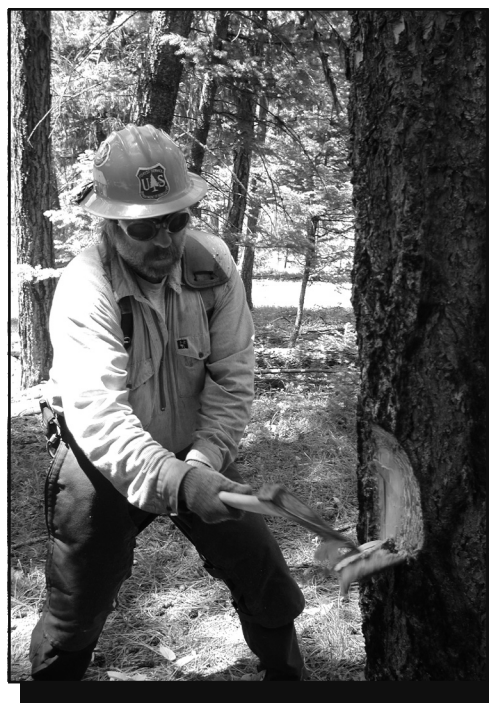
Figure 54—An ax can be used to remove bark from a log.
