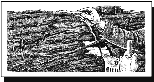
Figure 51 — A stick dropped into the kerf on a log with bottom bind will serve as a pivot when the log is cut through. This is a lost trick that is very practical and can prevent damage to the saw. — Now You're Logging , by Bus Griffiths, with permission of Harbour Publishing, Madeira Park, BC, Canada
