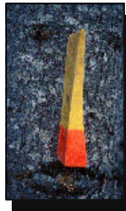
Figure 37—Triple-taper wedges allow a short wedge to provide as much lift as a longer wedge, but require more force to drive.
