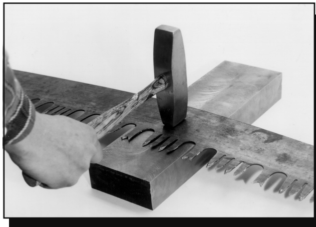
Figure 20—Hammering out a kink using a specially shaped saw hammer.
